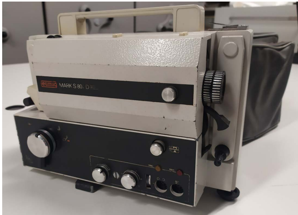
OBJECTE 3: projector Eumig model MARK S 807 D per a 8mm i Super 8
